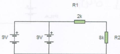
$$I_2 = I_1 = I_{PILA}$$
