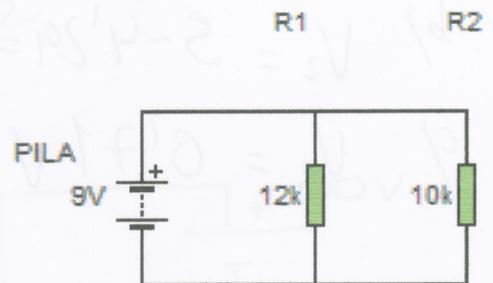
a)  $R_T = \frac{12 \cdot 10}{12 + 10} = \frac{120}{22} = 5'45\text{ K}\Omega$       $I = \frac{V_{PILA}}{R_T} = \frac{9\text{V}}{5454} = 0'00165\text{ A}$
