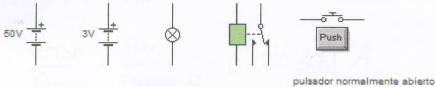
c)  $I_{\text{Bobina}} = \frac{V_{\text{PILA}}}{R_{\text{BOBINA}}} = \frac{3V}{35\Omega} = 0'085A$
